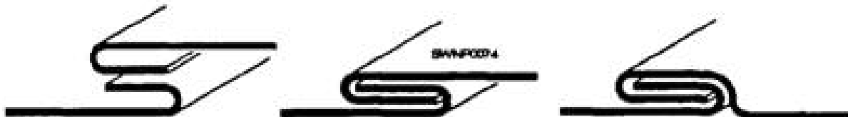
Figure 4: There are four S joints where the two long sides meet the two corner sides.
